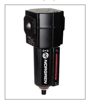
Ordering information. Models listed include PTF threads, automatic drain, metal bowl with liquid level indicator, and a 40  $\mu$ m element.
