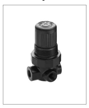
**Ordering Information.** Models listed include PTF threads, knob adjustment, non relieving diaphragm, 5 to 125 psig (0.3 to 8.6 bar) outlet pressure adjustment range†, and without gauge.
